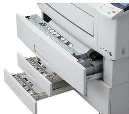
One roll of 3-inch core roll paper and two trays installed
